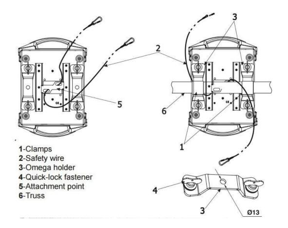
Use the spanner supplied with a projector to help installation.
