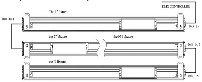
The connection of the signal amplifier(please note the wiring direction)
